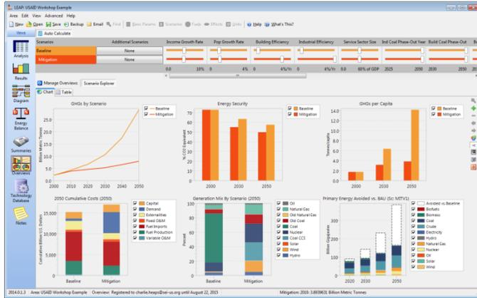
For example, a Low Emission Development Strategy (LEDS) might be modeled in LEAP, based on numerous separate Nationally Appropriate Mitigation Actions (NAMAs) in areas such as energy efficiency, fuel switching or renewables. Each NAMA can be individually modeled in LEAP as a scenario. These can be combined to explore which overall strategy is preferable with respect to costs, emissions reduction potential, energy security and national development objectives.
